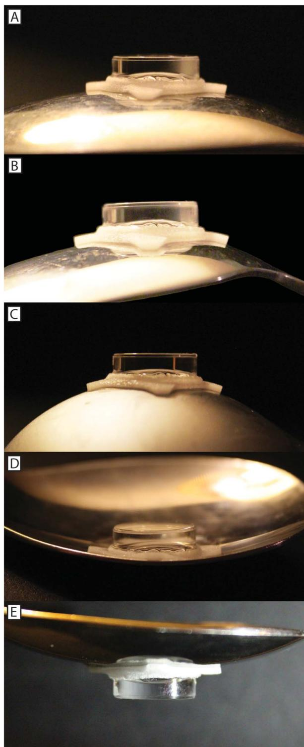
**Fig. 3.** Ex vivo demonstration of the ability of the absorbent sponge flange and legs to be able to conform to a variety of surface curvatures. The lens is seen conforming to and stabilizing on increasingly steeper convex surface curvatures of spoons (A–C). The lens' flexibility, stability, and adhesive properties even allow prolonged self-retention on concave surfaces (D) and upside down (E).
